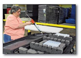
Pearl McNamar applies the glue for the last piece of specialized foam to be inserted in the case before it's packaged and shipped to customers.
